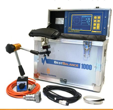
Best Balance 1000 is a portable device which is used for the measuring and the correction of the vibrations of rotating components due to the unbalance. It is designed for tools and machine tools but it may be also used to measure and correct the unbalance of other rotating bodies such as spindles, grinders, pulleys, rotors, fans, etc.
